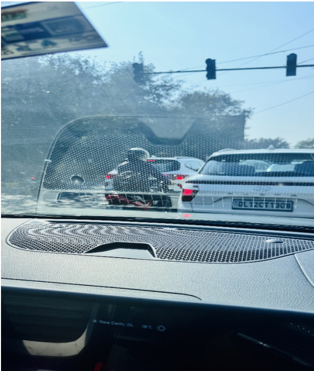
A real-world example of reflection-induced visual noise where dashboard textures are superimposed on the driver's forward field of view, reducing situational awareness.
